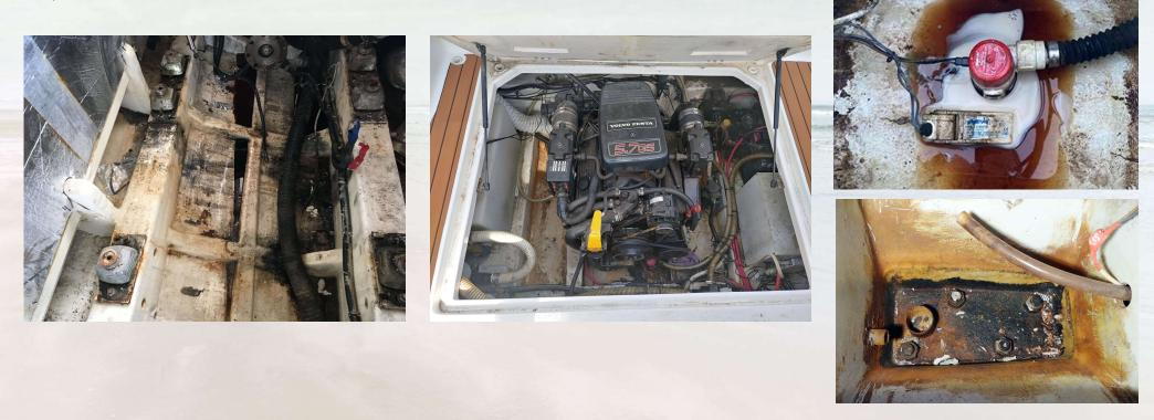
The bilge is amongst the most important places on the boat - one should thoroughly clean and inspect the bilge regularly especially during long trips.
