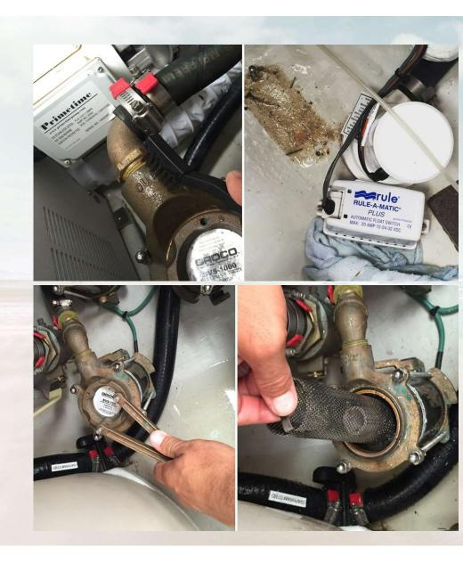
Use a wire brush to scrub any rust and corrosion of the brass and metal fittings. Be sure to inspect the unit itself for cracks and damage to the hoses.
