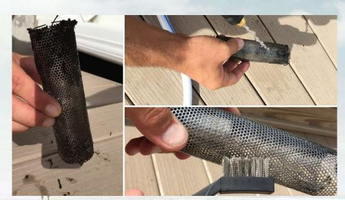
Scrub off any barnacles or corrosion with the wire brush, then reinstall and put the top back on. Remember to reset the seacocks to the proper position
